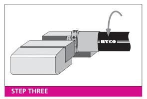
Screw anti-clockwise until hose bottoms in ferrule. Ease back between 1/2 and 3/4 of a turn.
