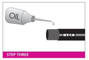
Lubricate exposed wire reinforcement.
