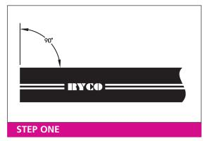
Cut hose to length required using a fine tooth hacksaw or cut-off saw. Ensure hose is cut squarely. Clean hose bore.
