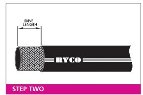
Mark Skive Length. (refer to Hose specification pages).Cut rubber cover around down to wire reinforcement. Slit lengthwise. Raise flap and pull off with pliers.
