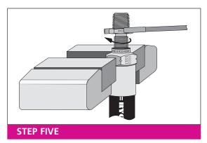
Screw insert clockwise right into ferrule using a continuous motion. Do not allow hose to turn during operation.
