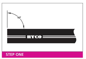
Cut hose to length required using a fine tooth hacksaw or cut-off saw. Ensure hose is cut squarely. Clean hose bore.
