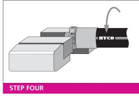
Screw anti-clockwise until hose bottoms in ferrule. Ease back between 1/2 and 3/4 of a turn.
